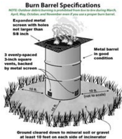
Specifications for a Proper Burn Barrel
